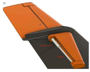
surface of the elevator. The control rod needs to be made of piano wire that is flexible enough to bend a little through the curve in the Bowden.
