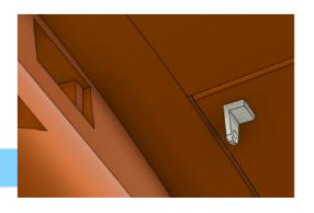
As the nacelles house the ESC's you should run a lead from the battery to the end of the wing. When assembled the esc should plug into this lead and the coupling should sit inside the end of the wing, not the nacelle.
