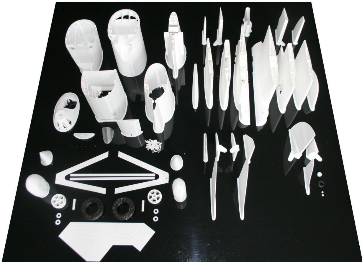
Figure 4: All printed parts at a glance
